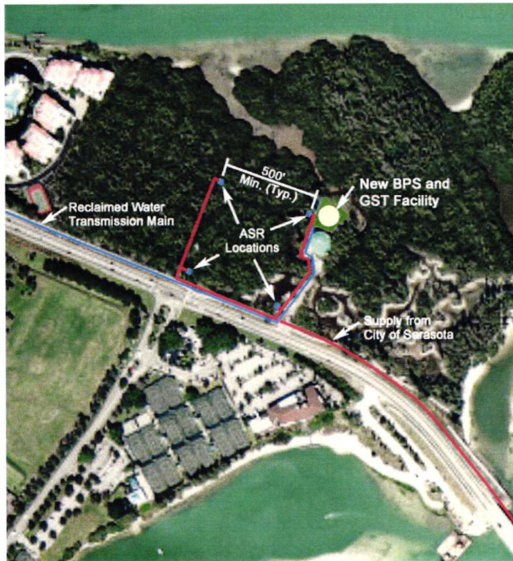
Figure 3-13 Conceptual Ground Storage Tank/Booster Pump Station Site
