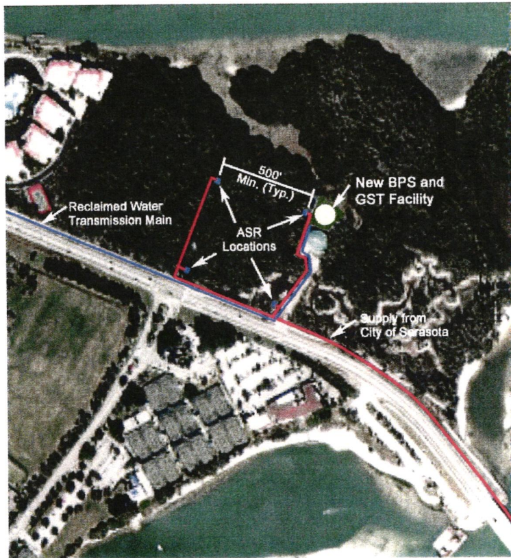
Figure 3-13 Conceptual Ground Storage Tank/Booster Pump Station Site
