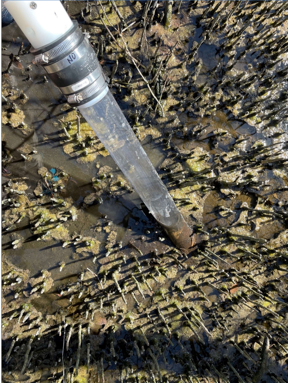
Figure 8 – Sediment corer with sample from sewage leak impact area.
