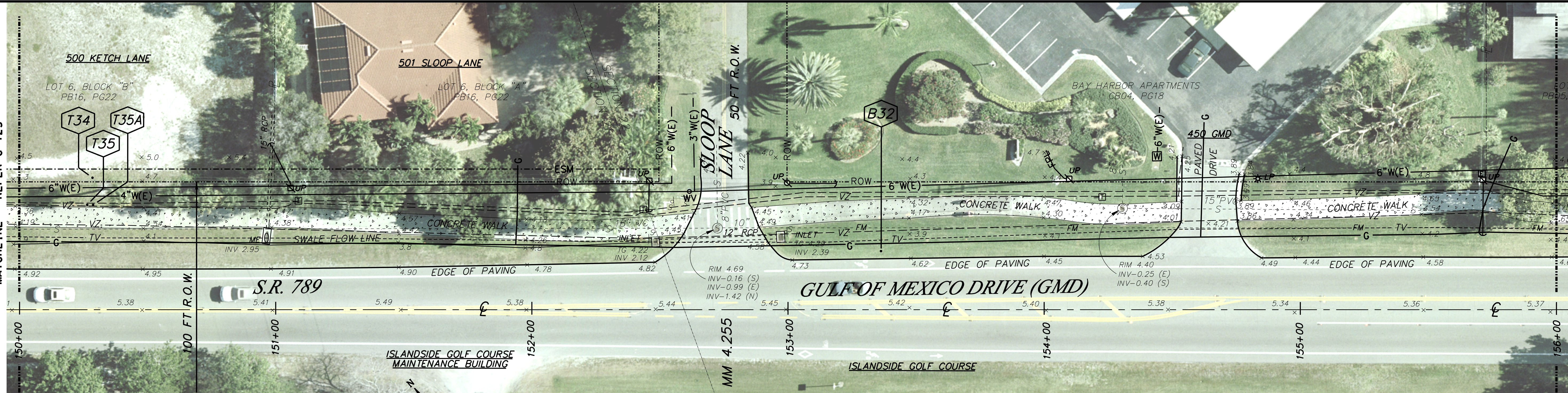
1 EXISTING ROADWAY, UTILITIES AND AERIAL STA 150+00 TO 156+00
