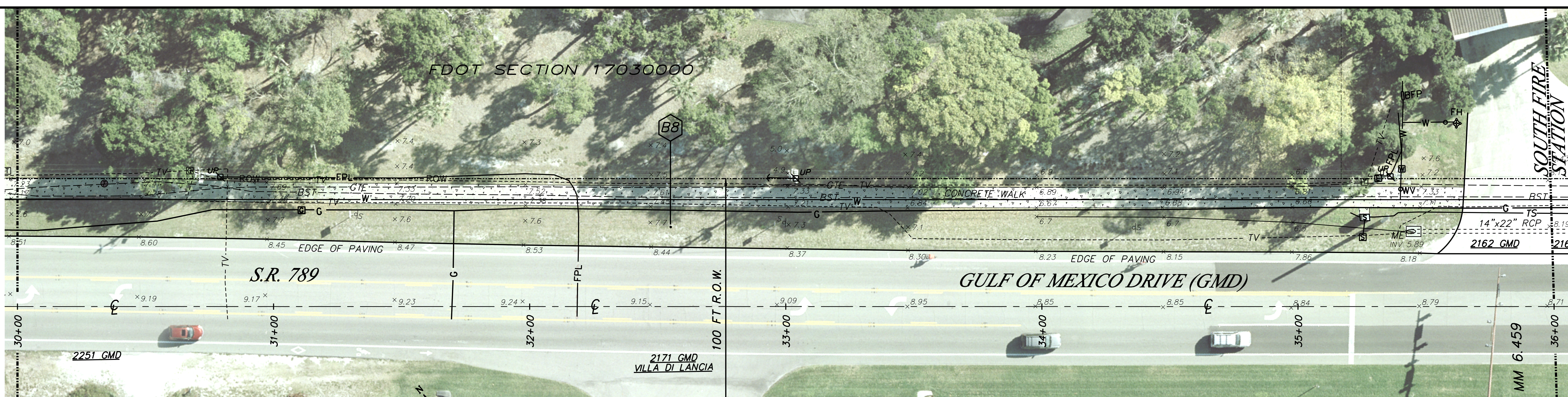
1 EXISTING ROADWAY, UTILITIES AND AERIAL STA 30+00 TO 36+00
