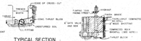
TYPICAL HYDRANT DETAIL
