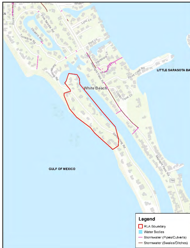
Figure 6: Distribution of Stormwater System Infrastructure
