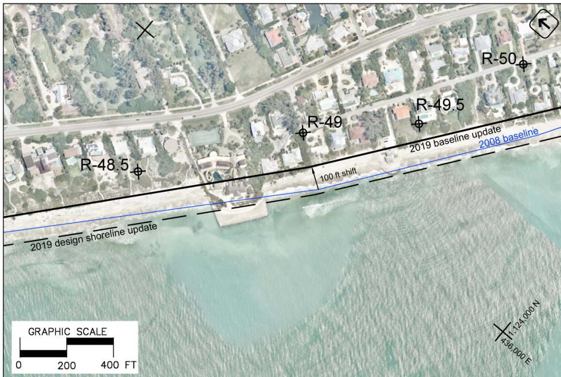
Figure 2.4 Updated baseline location in the vicinity of the 6633 Gulf of Mexico Drive seawall in Longboat Key, FL. The baseline was shifted 100 ft landward at R-49 in Manatee County.
