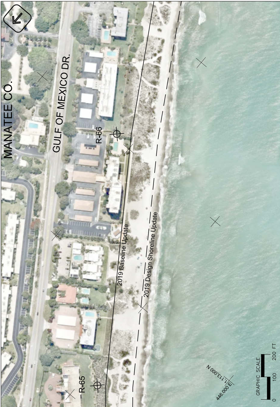
Figure A.15 2019 update to the baseline and design shoreline along the Longboat Key, FL, Gulf of Mexico shoreline (Photo Date: 7 May 2019).
