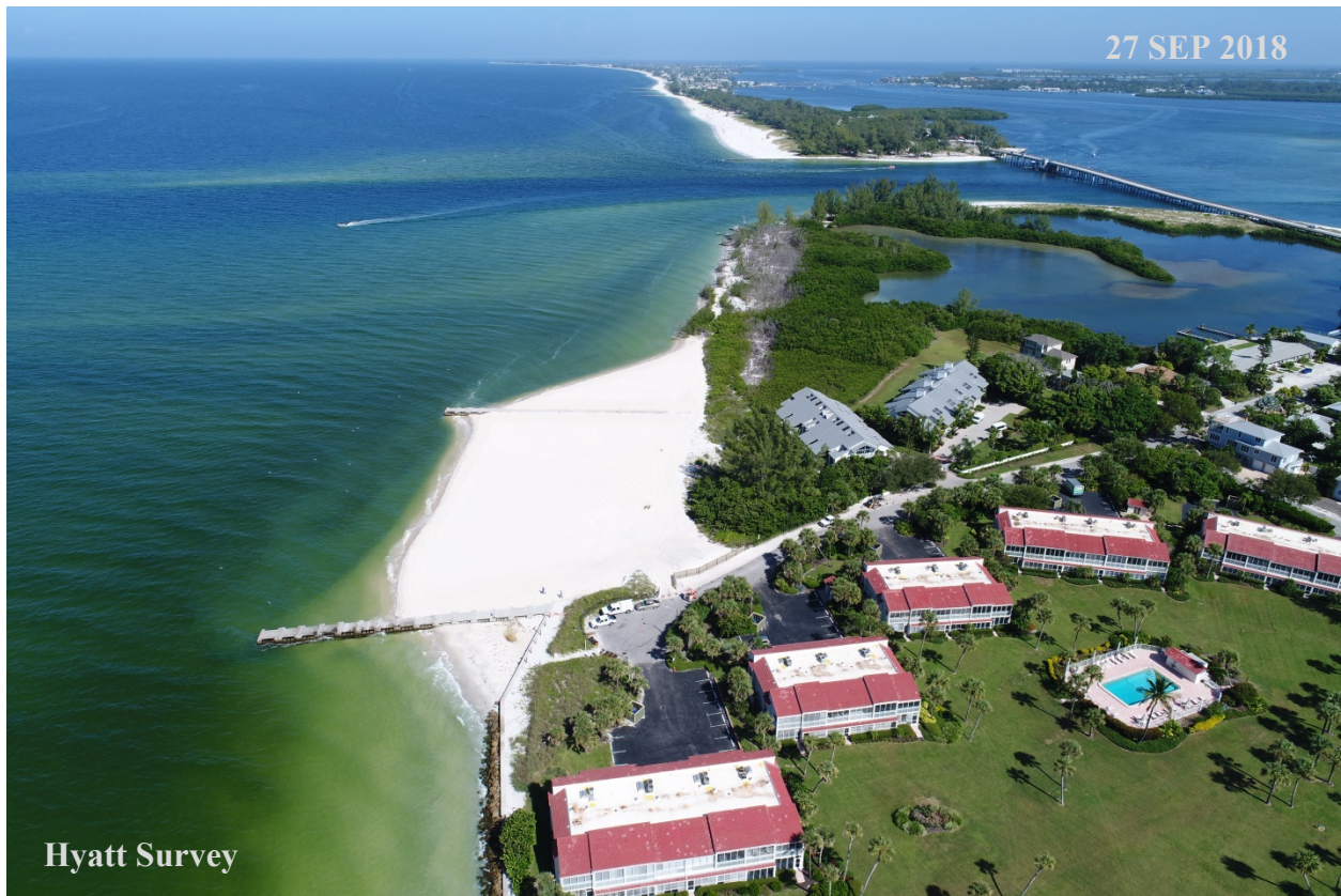
Figure 5.7 The condition of the beach immediately following the 2018 North End Interim Beach Nourishment Project at North Shore Road in Longboat Key, FL. Sand for the project was sourced from CEMEX Davenport.
