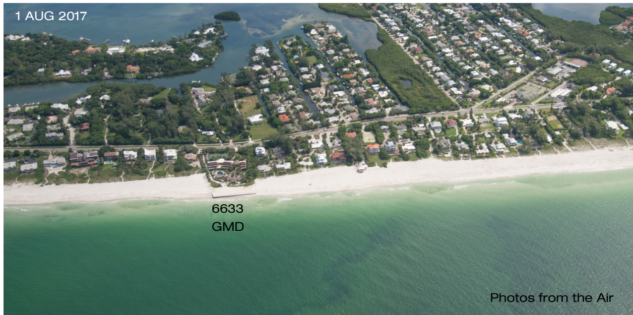
Figure 3.4 A comparison of beach conditions in the vicinity of the 6633 Gulf of Mexico Drive seawall immediately post-construction (top frame) and nearly one year (bottom frame) following the 2016 Longboat Pass Dredging and Beach Nourishment Project. Maintaining the design MHW shoreline that was located 120 ft Gulfward of the seawall (CPE, 2008) has proven to be infeasible.
