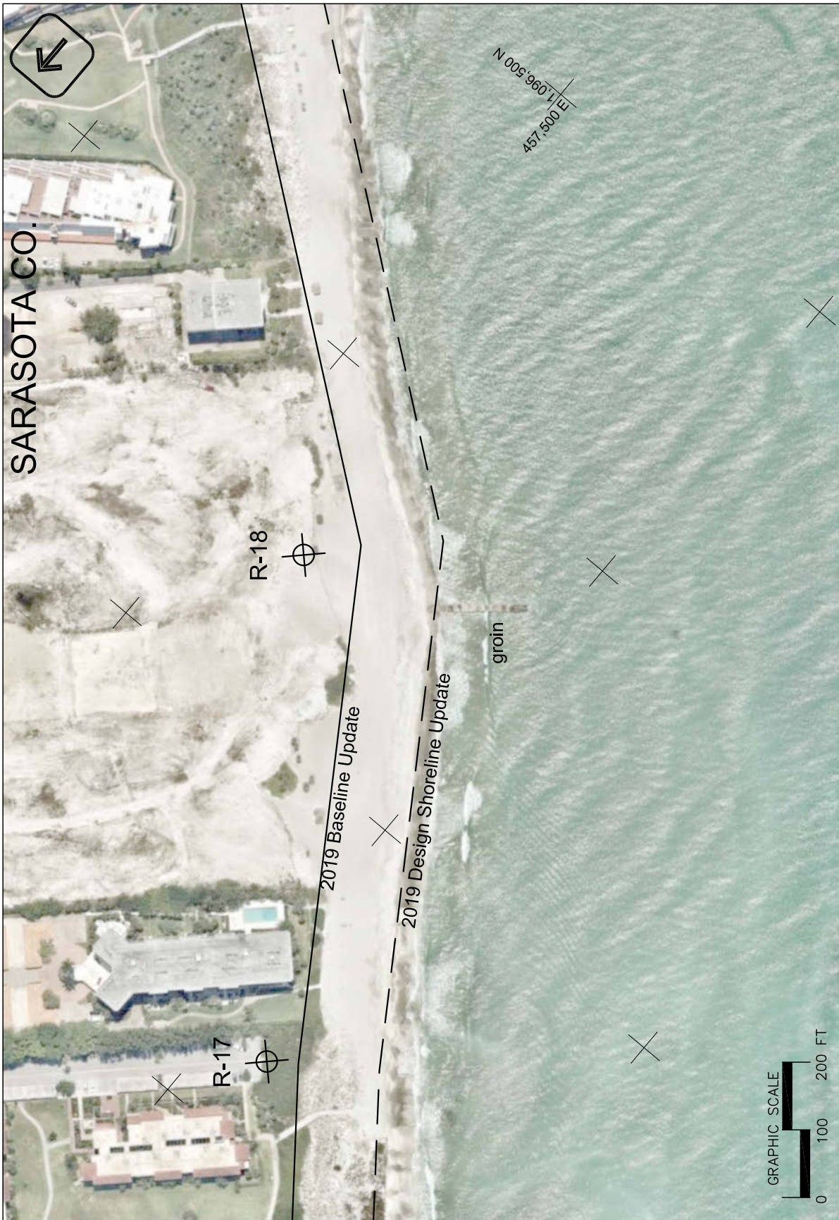
Figure A.27 2019 update to the baseline and design shoreline along the Longboat Key, FL, Gulf of Mexico shoreline (Photo Date: 7 May 2019).
