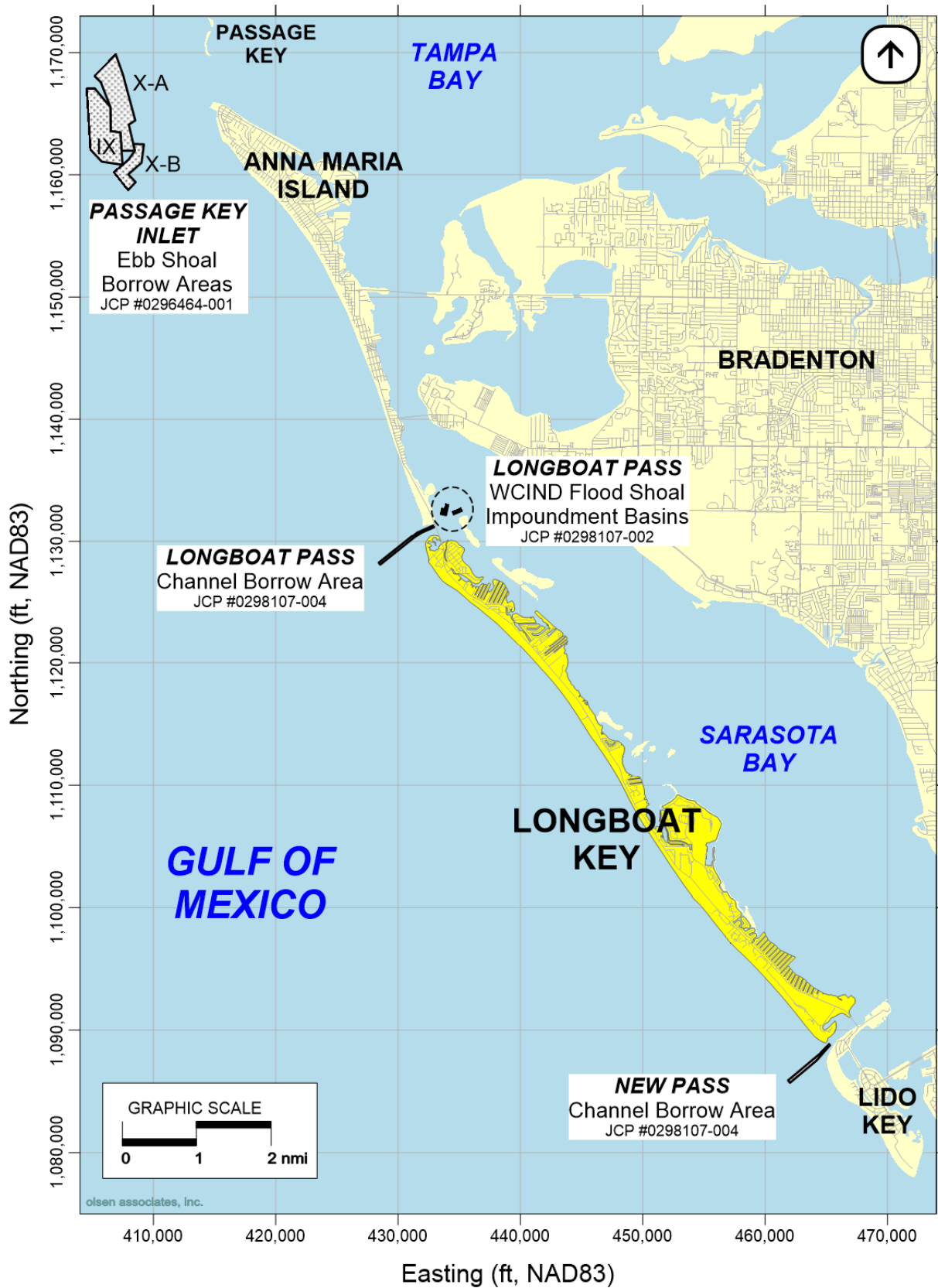
Figure 4.2 Location map of permitted inlet borrow areas for Longboat Key beach nourishment
