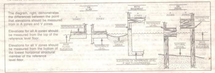
The reference level elevation may be reported to the same level of precision used to report base flood elevation on the FIRM (e.g., if the base flood elevation is shown to the nearest half foot, the reference level may be reported to the nearest half foot).
