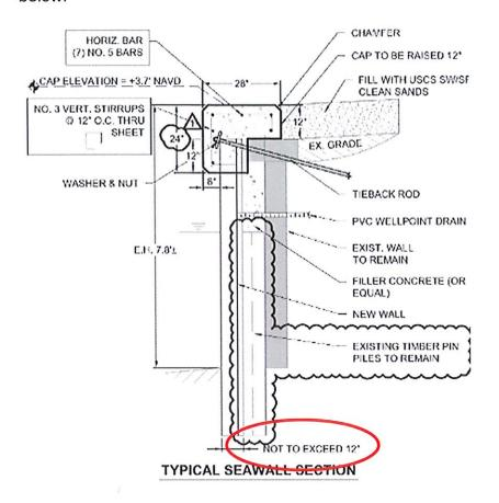
4. April 11, 2024. Revised Change Order plans submitted. Change Order requested landward-oriented modification to the seawall cap *only*, by adding 8 inches to the overall width of the seawall cap increasing the cap to 36" in width (Section view detail provided below). (Note: Building permit application did not depict nor include seawall construction occurring at 592 Ranger Lane).
